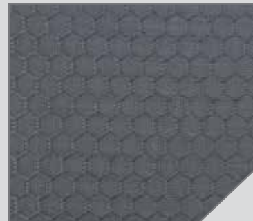
500D Hex Ripstop Nylon Fabric with Teflon® Coating
